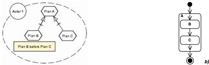
Fig. 5. A Tropos plan AND-decomposition diagram with temporal annotation for a given Actor and the corresponding UML 2.0 activity diagram
