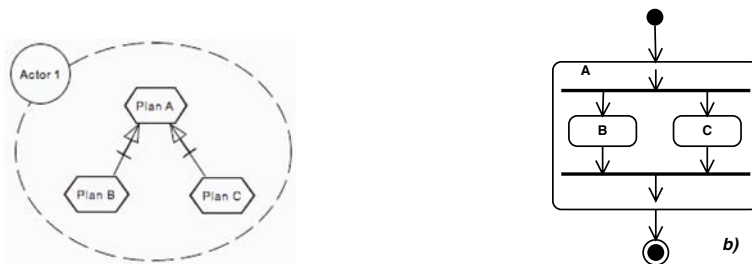
Fig. 3. A Tropos plan decomposition diagram for a given Actor and the corresponding UML 2.0 activity diagram
